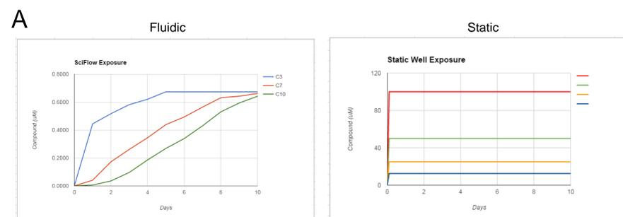
In an acellular scenario (A), SciFlow (left) dosing creates gradients of compound concentrations over time. The concentration of compound increases in each well until the equilibrium concentration is reached, and then that concentration is maintained for the duration of the experiment. Wells at different distances from the source well have very different concentration exposure profiles. Static plates (right) are at a fixed concentration, which only varies due to cellular metabolism.
