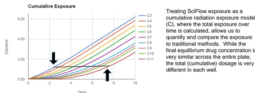
Treating SciFlow exposure as a cumulative radiation exposure model (C), where the total exposure over time is calculated, allows us to quantify and compare the exposure to traditional methods. While the final equilibrium drug concentration is very similar across the entire plate, the total (cumulative) dosage is very different in each well.
