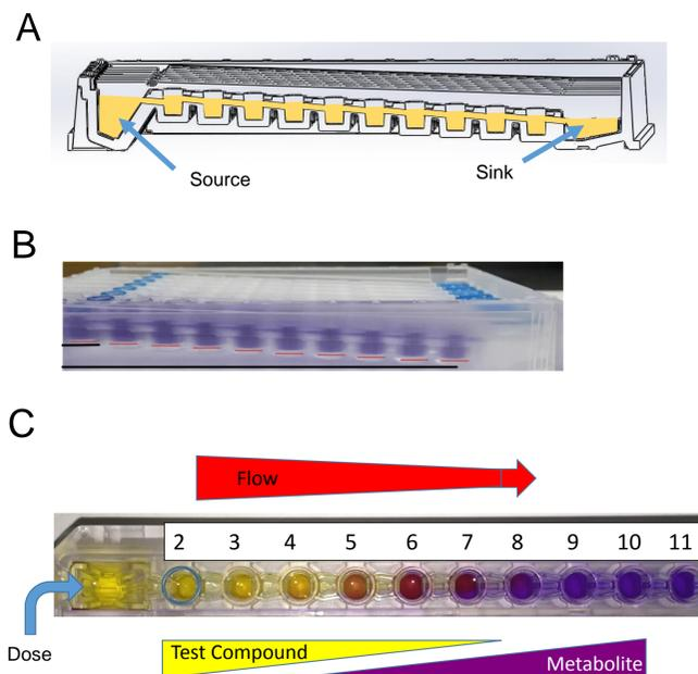
Panel A shows a schematic side view of SciFlow with the source and sink wells identified 0.5mm decrease in height for each well bottom. Panel B is a picture of SciFlow, with purple liquid filling one row to highlight the 0.5mm decrease in Z-height (height of well bottom) across the plate. Panel C is a top down view of one SciFlow row highlighting the dual gradients of decreasing parent compound and increasing metabolite down the row.
